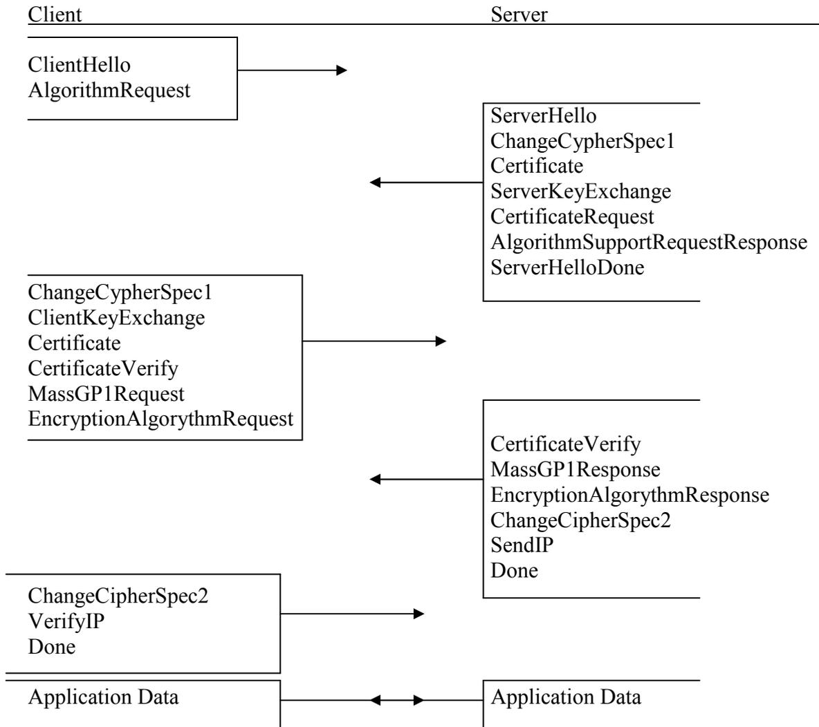
Figure 3.2 Modified 4-Way TLS Handshake
